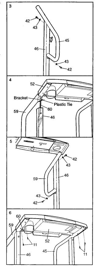
7. Make sure that all parts are tightened before you use the treadmill. Keep the included allen wrench in a secure place. The allen wrench is used to adjust the walking belt (see page 13). To protect the floor or carpet, place a mat under the treadmill.
